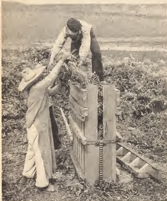
After weighing, the shrub is pressed into 100-pound bales by means of this ancient baling machine.
